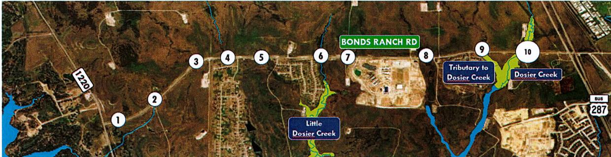
Two of the ten drainage crossings are located within FEMA Zone A floodplain and the remainder are unmapped. A floodplain analysis will be performed for all crossings in accordance with City of Fort Worth Standards and the minimum requirements of the National Flood Insurance Program (NFIP) as administered by the Federal Emergency Management Agency (FEMA). A LOMR has been scoped below for the two crossings within FEMA floodplain.
